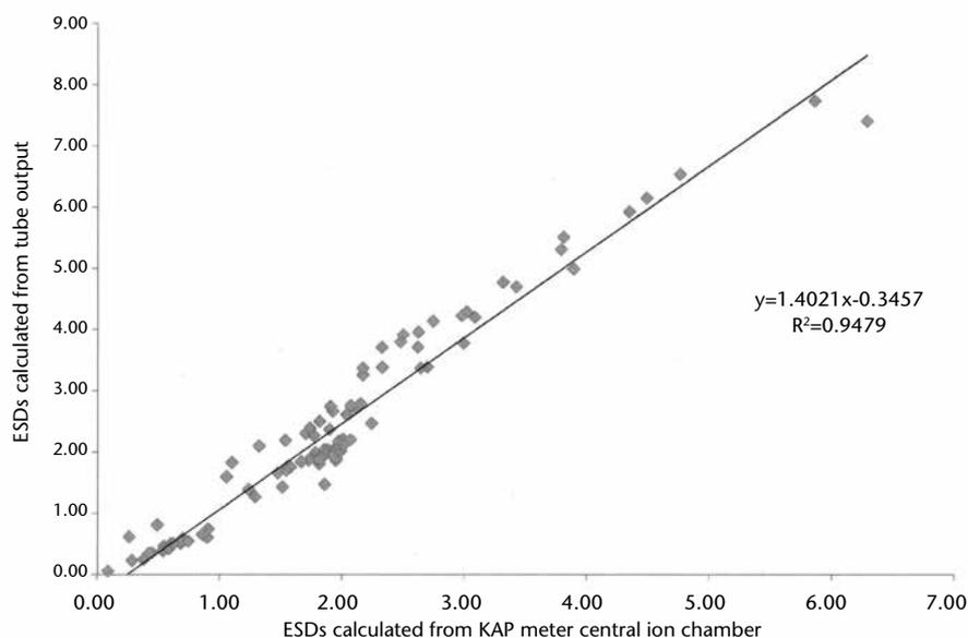
**Figure 2.** The entrance surface doses (ESD) calculated from tube output vs. the value calculated from reading for the central ion chamber of the kerma area product (KAP) meter for the anteroposterior kidney-ureter-bladder radiography examinations. The correlation coefficient ( $R^2$ ) between the data sets was 0.9479.
