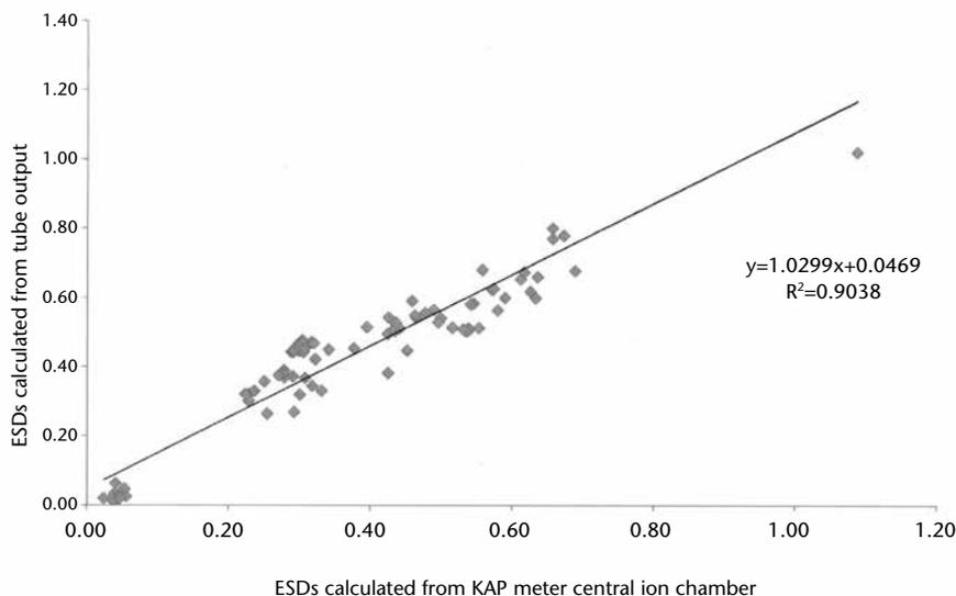
**Figure 1.** The entrance surface doses (ESDs) calculated from tube output vs. the value calculated from reading for the central ion chamber of the kerma area product (KAP) meter for the posteroanterior chest examinations. The correlation coefficient ( $R^2$ ) between the datasets was 0.9038.
